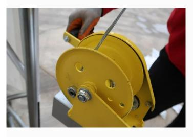
10. Turn the winch clockwise to lift the door curtain cloth and bracing tubes to a position about 40-50cm away from the cross beam. Lace the eyelets on the cloth to cross beam with a rope. Refer to Figure 5.
