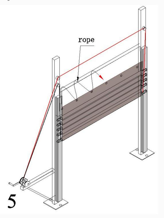
11. Now the winch door installation is completed. Turn the winch clockwise to raise and counterclockwise to lower the door. The steel wire rope shall be evenly wound on the winch so that the door can rise and fall smoothly.
