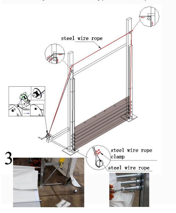
9. Adjust the length of the steel wire rope to be equal on both sides. Fix the wire rope fold to the hole in the winch. Refer to Figure 4.
