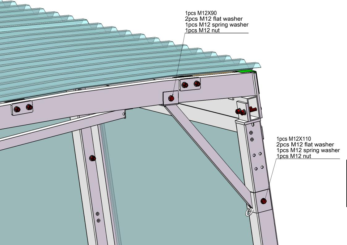
There are 12pcs inclined supports without ring. Every post need install one inclined support
