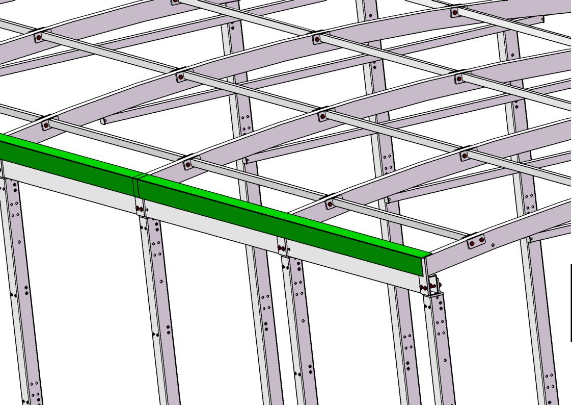
Put the corrugated FRP plate on the top. Connect with the self-tapping screws
